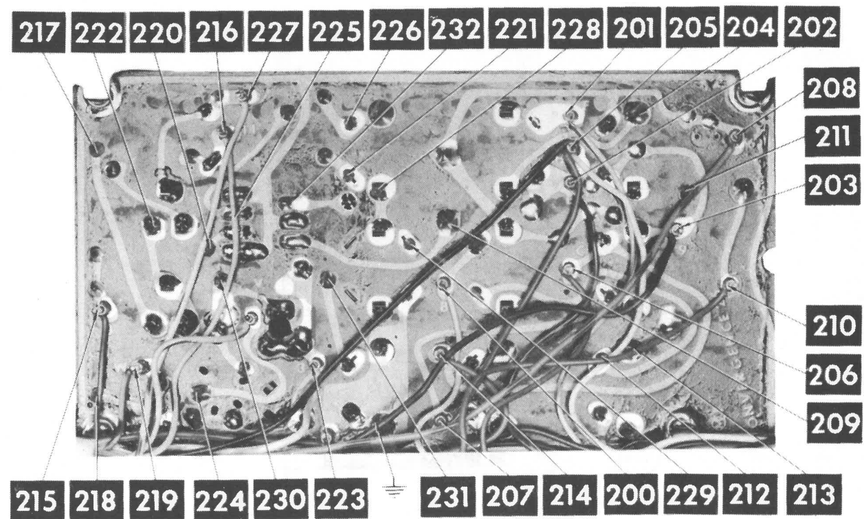
A Howard W. Sams CIRCUITRACE® Photo CONVERGENCE BOARD
