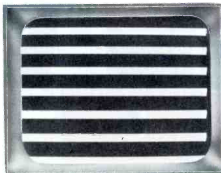
Fig. 1. Horizontal-Bar Pattern Produced on Screen Is Caused by Audio Modulation of RF Generator.
