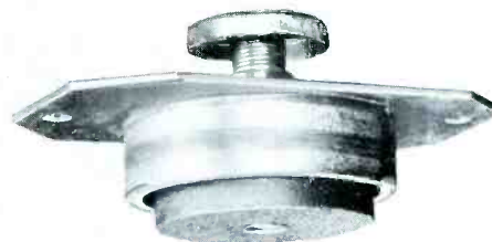
Fig. 9-39. One of the Rim Magnets Used in the RCA Victor Model 21CT55.
