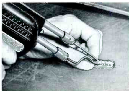
Fig. 13. Curing a Cold Solder Joint on a Tuner Strip.
