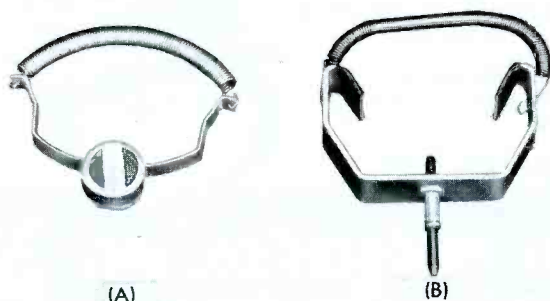
Fig. 9-45. Lateral-Correction Devices Used in (A) RCA Victor Model 21CT55 and (B) Motorola Model 19CT1.
