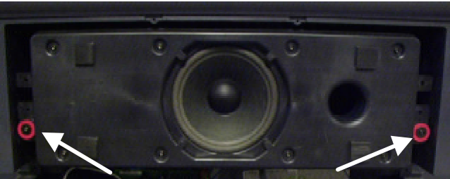
Screws Securing Subwoofer
