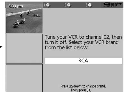
When the GUIDE Plus+ Gold System correctly identifies the correct code for your VCR, the VCR's tuner changes to channel 9. Select *YES* if the VCR automatically changed to channel 9, or *NO* if it did not. If you select *NO*, the system will try another code.
