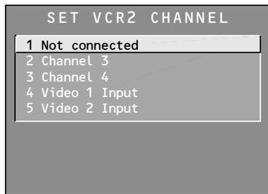
2. Point to the choice that matches the way you have your second VCR connected to the TV. If you used audio/video cables, choose the video input you connected the cables to.
