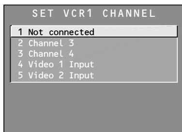
2. Point to the choice that matches the way you have your VCR connected to the TV. If you used audio/video cables, choose the video input you connected the cables to.
