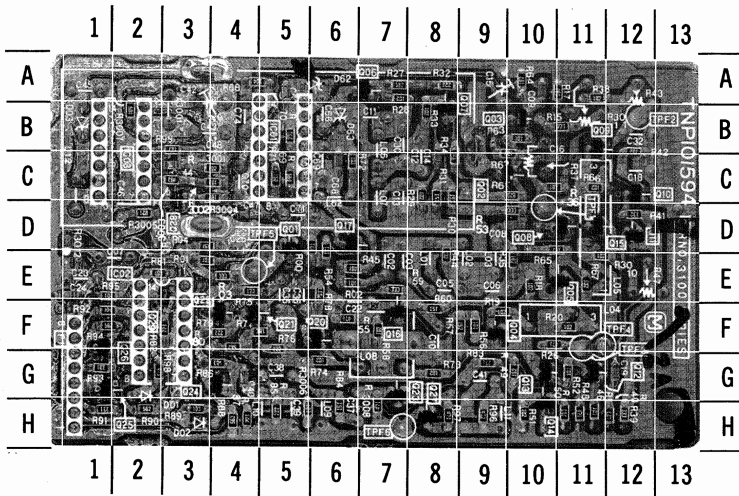
A HOWARD W. SAMS GRIDTRACE™ PHOTO COMB FILTER BOARD-BOTTOM VIEW
